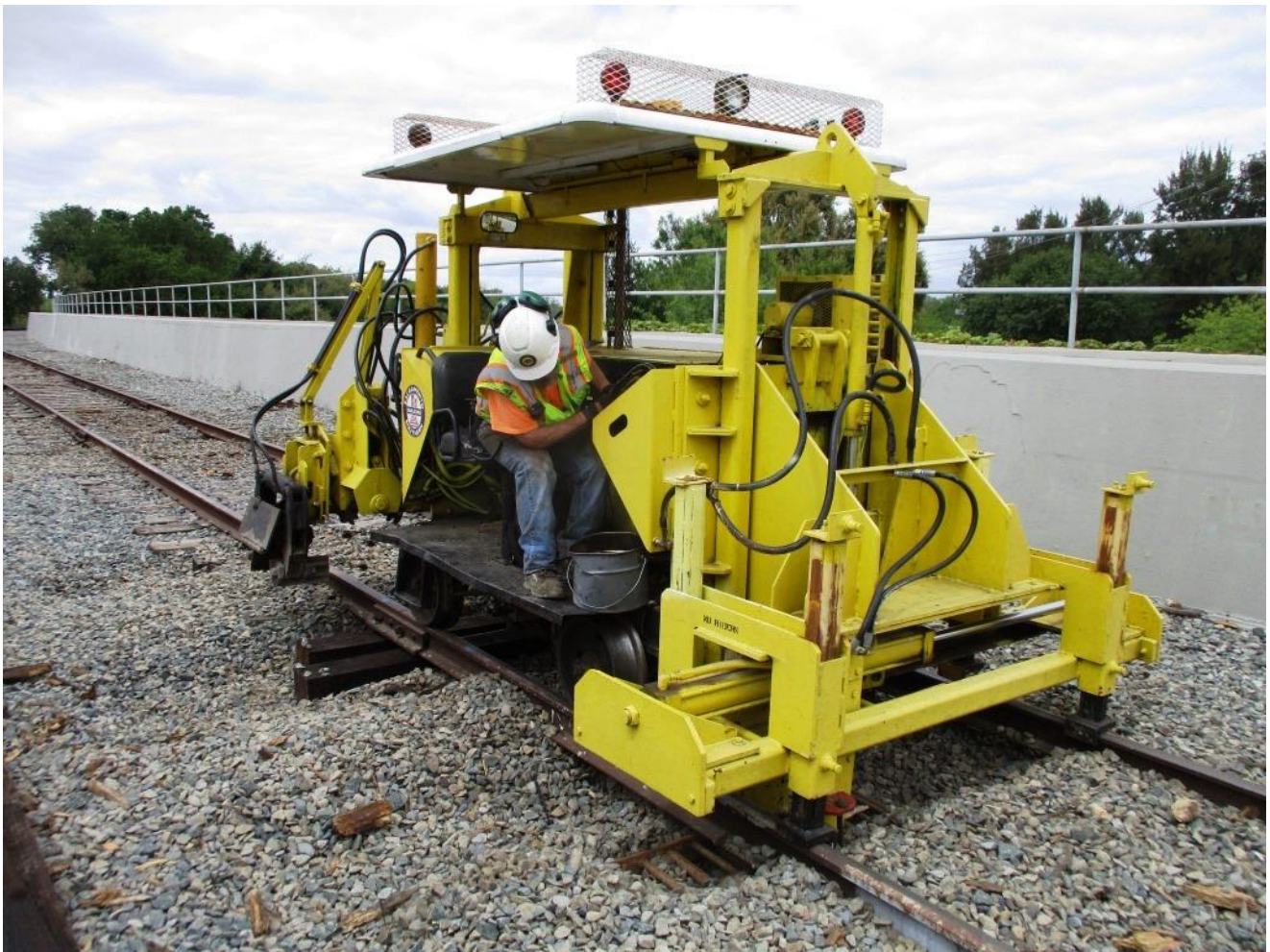
Joe employs the rarely used scarifier function on the 125 to provide a little more depth under the rails at this tie-crib
