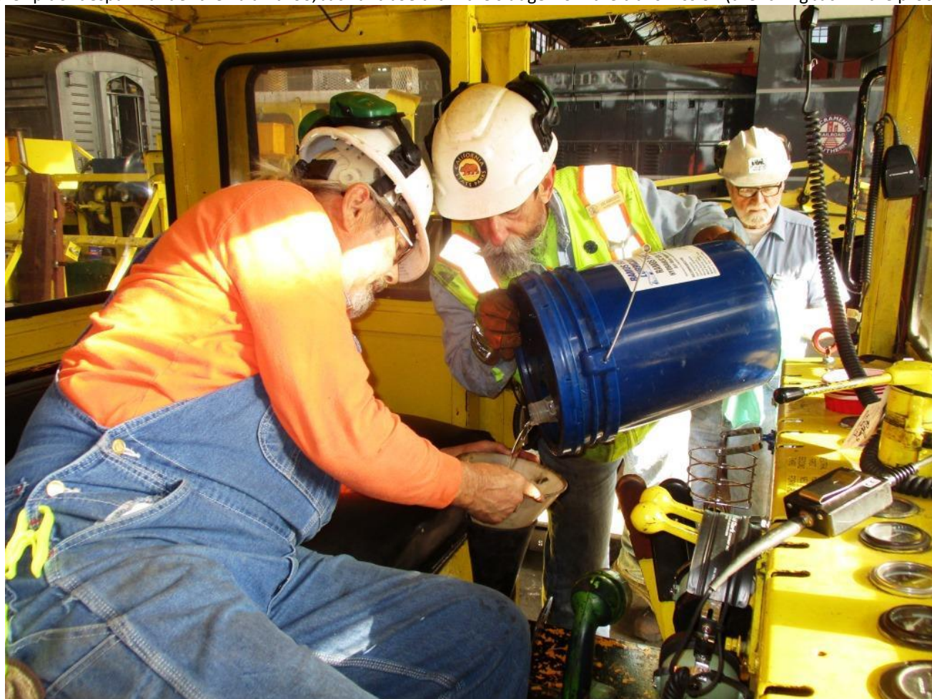
With all the sludge gone, Ed and Joe fill the transmission with fresh hydraulic fluid
